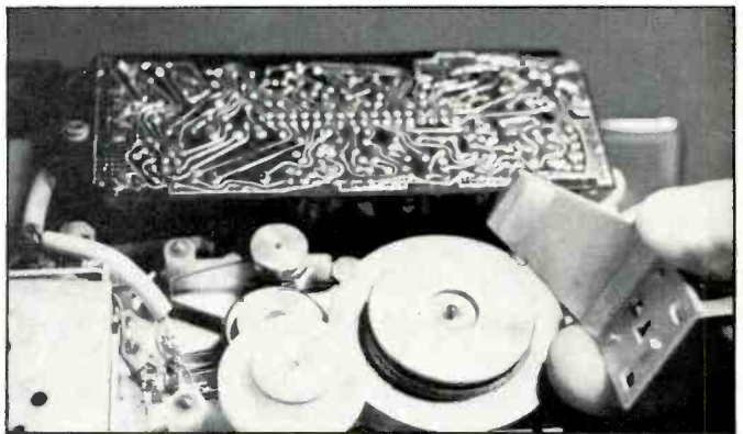
Fig. 7—Showing the underside of the deck, with main-drive belt and lower flywheel bearing removed.
