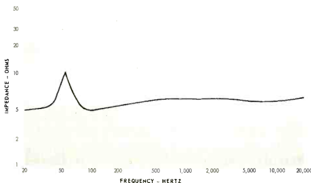
Fig. 5—Impedance characteristics of "Project M" system
