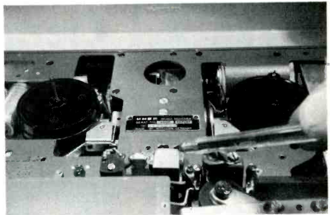
Fig. 6—Uher 4000 allows very little access for cleaning and is better served by an impregnated cleaning band.
