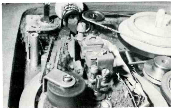
Fig. 1—"Loss of tape contact seriously affects the response." This Grundig deck collected so much dirt it was a wonder it played at all!
