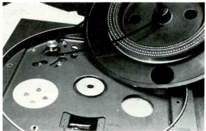
Fig. 3 —Looking down into the turntable's drive motor pulley reveals the drive elements. The motor pulley (top) drives the underside of the platter, which is removed and turned over (right-hand corner), via a neoprene belt. Strobe markings may be seen on the platter, as well as a balance weight. The strobe lamp can be seen at bottom.
