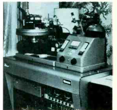
Gotham Audio displayed an operating Neumann disc-cutter that cut an LP master from a master tape played on a Studer tape machine.
