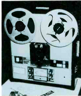
3M film-sync two-track recorder, with one track for audio and one for the sync signal.
