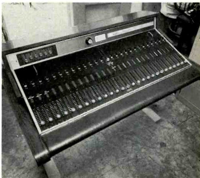
Fig. 3—View of the Altec 9200 console, custom built for the Greek Theatre. Should expansion be required at a later time, different strip modules can be installed.
