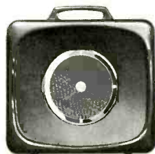
Electro-Voice "Sonocaster I" —8" coax. spkr. in molded housing, 8 ohms, handles 30 watts (peak), 70-13 kHz, 16 3 / 4 " x 17" x 5 5 / 8 ", 6 3 / 4 " lbs., $25.00.
