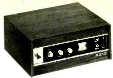
Fig. 1—Sony's Model 230 "Stereo Compact," a portable 4-track stereo record/playback tape system with a stereo control center, is shown at left. It's also available as Model 230W in a walnut cabinet, as shown above. Matching walnut bookshelf speakers (not shown) are optional.
