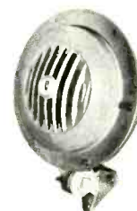
University Sound MM-2PPS —Underwater spkr., 16 ohms, handles 25 watts (music power), 100-10 kHz, 7 3/16" diam. x 3 3 / 8 ", 5 1 / 4 lbs., $46.50.
