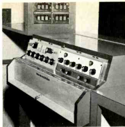
Fig. 5—Control console and part of the rack-mounted cabinet which houses amplifiers are shown here. Switches on panel control lights.
