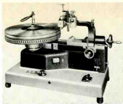
Fig. 3—Example of a disc mastering lathe, the Neumann AM-131, shown with a Neumann ES-59 mono dynamic feedback cutterhead mounted.
