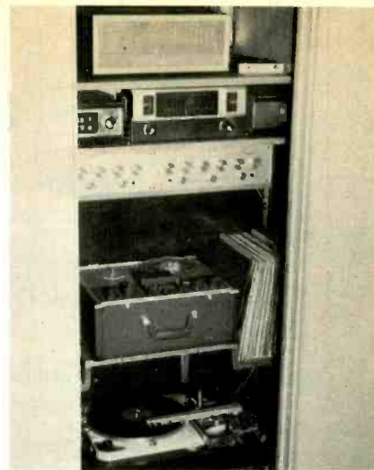
Fig. 5—The author's present system includes the following components: ADC 10E stereo cartridge in a special moving-pivot tone arm; Thoren TD-124 manual turntable; Ampex 1260 4-track tape recorder; Marantz mono preamplifiers; Knight AM tuner; Fisher FM tuner; Marantz electronic crossovers at 100 Hz and 3500 Hz; JBL N-500 crossover networks at 500 Hz; Eico 28-watt dual basic amplifier above 3500 Hz; Marantz 40-watt basic amplifiers between 100 Hz and 3500 Hz. The latter drives JBL theatre woofers to 500 Hz and Stephens P-35 theatre drivers above 500 Hz. A Marantz 40-watt basic amplifier drives an Electro-Voice 15-in. "K" horn; Ionovac tweeters and JBL high-frequency lenses round out the system.
