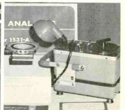
Bruel & Kjaer exhibited test instruments, including a new tape recorder for lab measurements. General Radio showed how its Strobotac (electronic stroboscope) stopped motion of a speaker's vibrating cone so that its movements can be analyzed.
