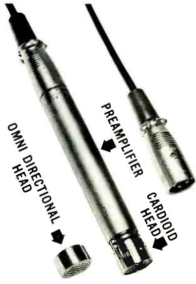
Fig. 9—Some condenser microphones offer the flexibility of changing heads from omnidirectional types to unidirectional types and vice versa.
