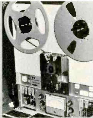
The 3M Co.'s "Isoloop" professional tape recorder with front panel removable printed circuit boards.
