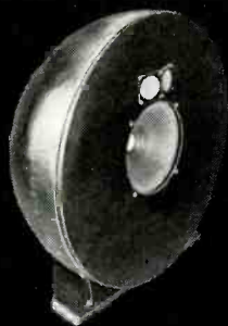
1949 First product of the newly formed Bozak company was the Model B-201, aptly named the "kettle drum" from its 32-inch hemispherical steel infinite baffle enclosure. Its honest frequency response from 40 to 13,000 cycles would do credit to many modern systems.
