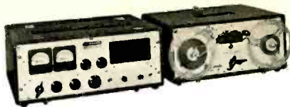
The well remembered Magnecord PT6-JA, comprising the recorder, together with amplifier and speaker.
