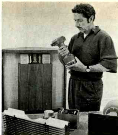
Bill Hartsfield putting the finishing touches to a JBL speaker system that bears his name. Note use of acoustic lenses.
