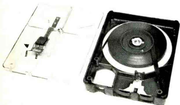
Fig. 1. The Fidelipac tape cartridge with cover removed.
