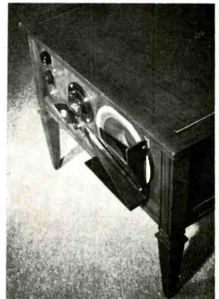
Fig. 3. Looking down on the rear of the end-table speaker to show one type of reflector in front of the midrange cone.
