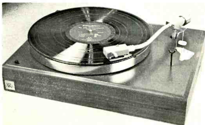
Fig. 5. An AR turntable with an anti-skating device built-on consisting of a bent paper clip held in place with tape. A small piece of thread and a plastic gram weight complete the assembly.
