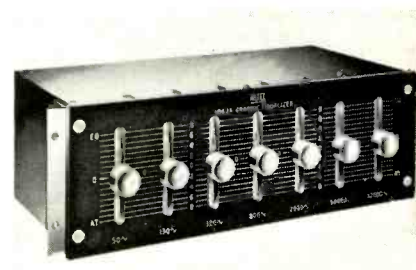
Fig. 30. Graphic Equalizer which will permit boost or cut of 8 dB at any of seven frequencies approximately 1\frac{1}{2} octaves apart. One, two, three, or all of the controls may be varied to achieve the desired effect.
