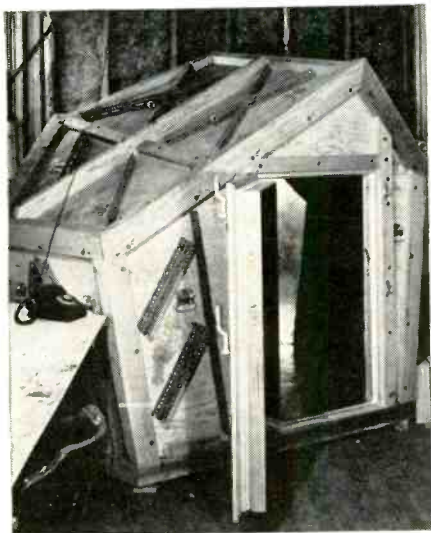
Fig. 5. AR's reverberant chamber for speaker testing.
