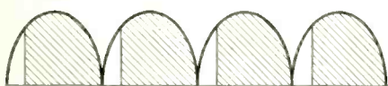
WHEN SCR IS FIRED EARLY IN THE CYCLE, THE LAMP IS PASSING CURRENT FOR MOST OF THE CYCLE AND THUS IS BRIGHT
