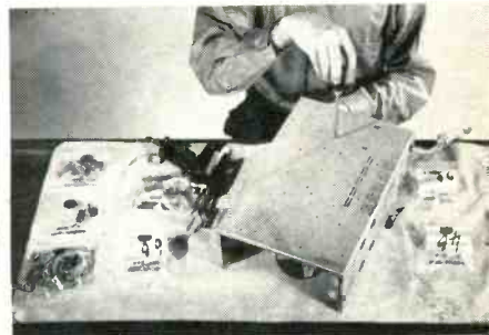
The cloth makes an excellent work surface since small bits of hardware and tiny electronic parts won't roll or slide off it. Tricky-to-wire parts of the circuitry come pre-assembled on plug-in printed-circuit boards.
