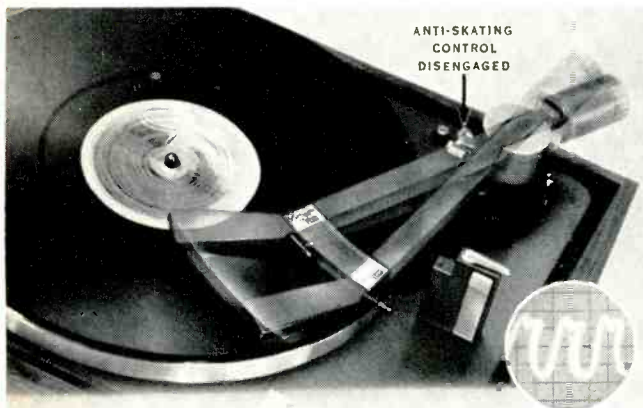
4 "Now you can actually watch the strength of the skating force. I start the Lab 80, but flip the anti-skating control over and out of operation. Note that as soon as I put the stylus on the grooveless record, the arm moves rapidly... with force, toward the center."
