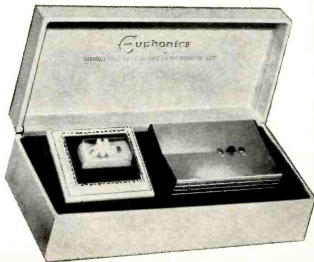
Fig. 4. The Euphonics CK-15-LS Phono Cartridge and its power supply.
