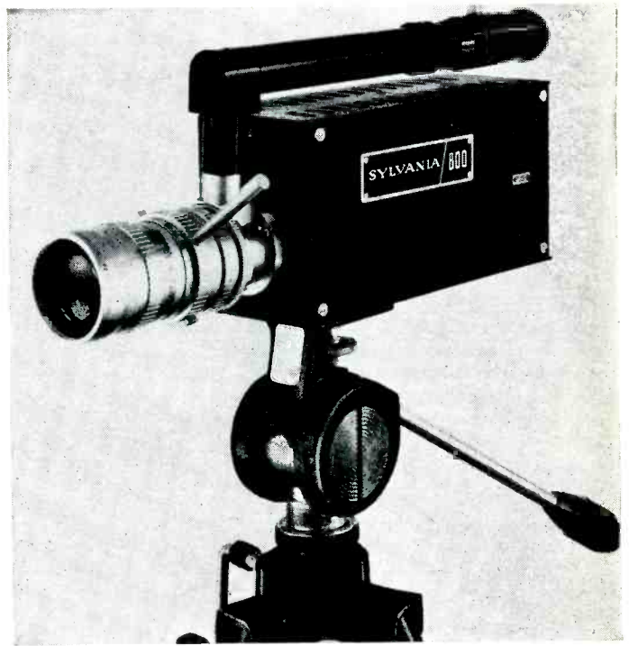
The recently released Sylvania vidicon camera with a 4 to 1 Angenieux zoom lens.
