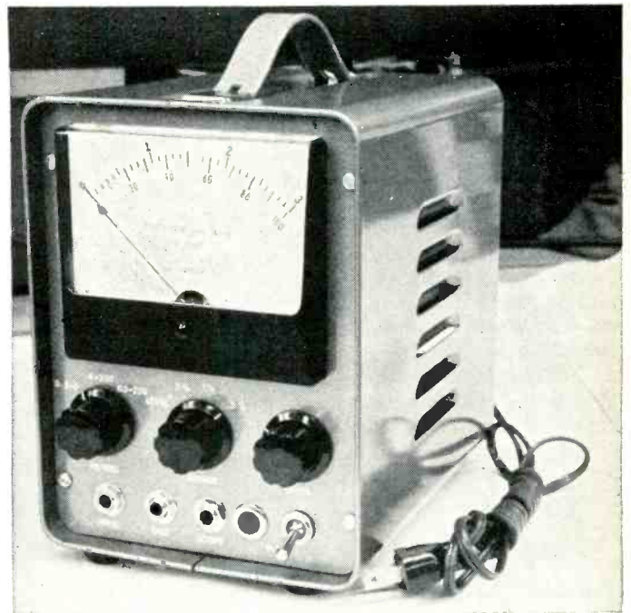
Front view of the author's flutter meter.
