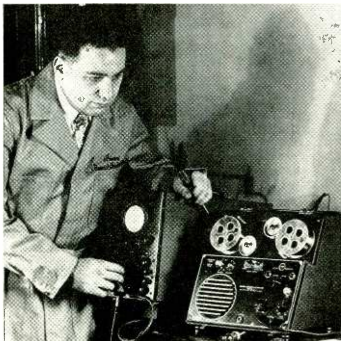
Fig. 1. The wire recorder shown here is one of hundreds made by Armour Research Foundation during World War II for the U. S. Armed Forces. At left is Marvin Camras, who developed and patented the machine in 1939. (1943)
