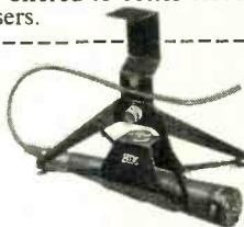
ALTEC 685A CARDIOID MICROPHONE SHOWN IN ALTEC 181A BOOM MOUNT Frequency Response: 40 to 16,000 cycles • Output Impedance: 30/50, 150/250, 20,000 ohms • Output Level: -54 dbm/10 dynes/cm 2 • Discrimination: Average front-to-back, 20 db • Hum: -120 db (Ref.: 10 -3 Gauss) Price $96.00 net
