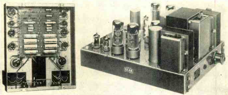
Fig. 1. Leak Stereo 60 power amplifier showing top and under-chassis views. Note military-board construction.
