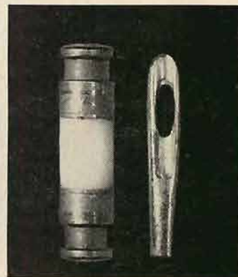
Heart of amplifier—a hermetically sealed gallium arsenide diode—is compared with eye of average-sized sewing needle.
