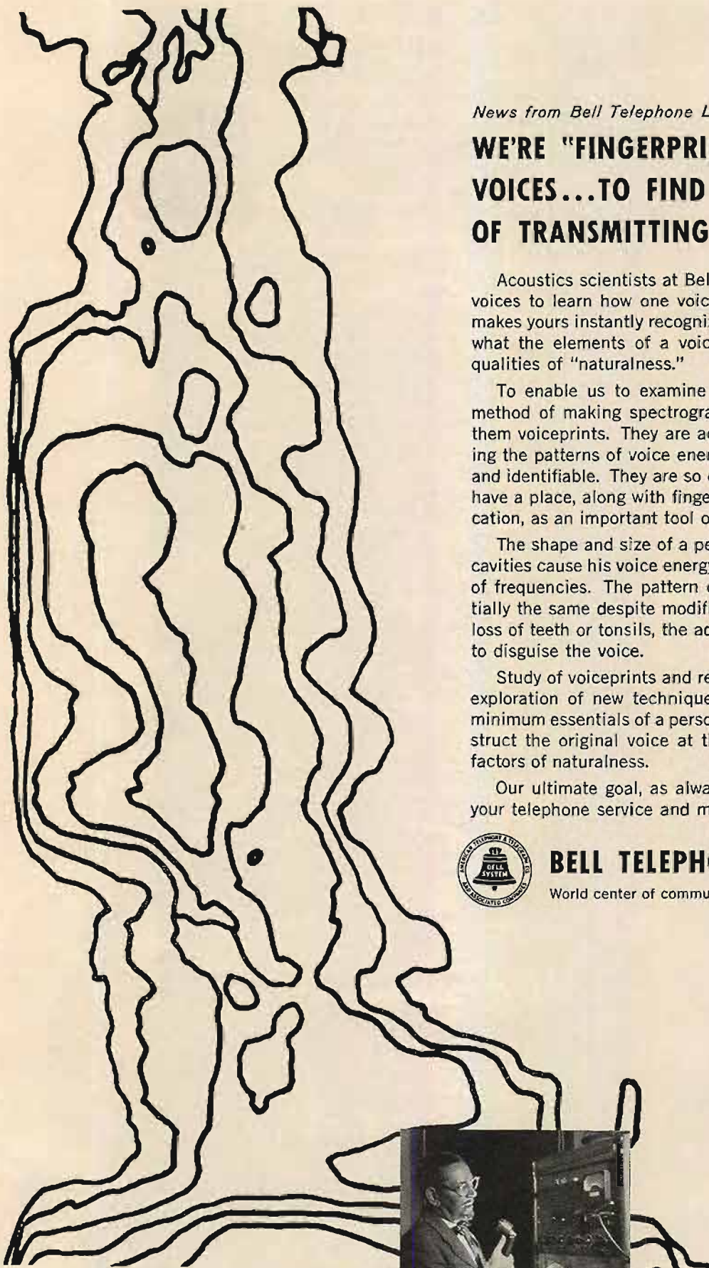
Word Picture. This is a picture of the spoken word "you." By analyzing the sound with a spectrograph, the Laboratories' Lawrence G. Kersta makes a print of the word in graph form. Graph shows frequency, time taken, and intensity used in making speech sound.
