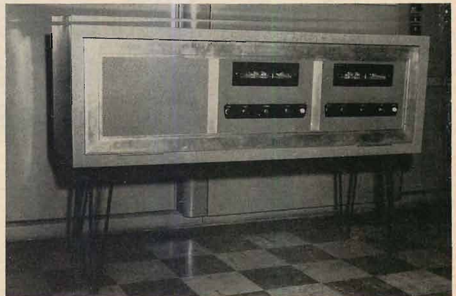
Fig. 19. Three playback decks can be put in one cabinet. The front door folds down on this cabinet too.
