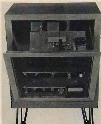
Fig. 18. The equipment is housed in a mica-covered plywood cabinet. Its front door drops down part way for convenient weekly maintenance. It opens all the way for major servicing problems.
