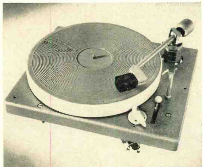
Fig. 5. Neumann automatic 2-speed integrated turntable.
