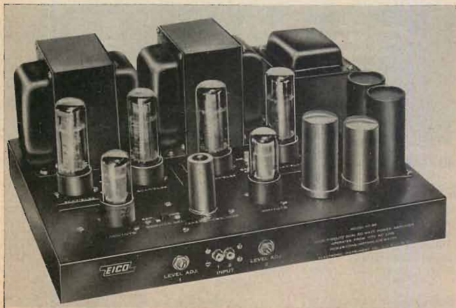
Fig. 1. EICO Model HF-89 dual 50-watt stereo power amplifier.
