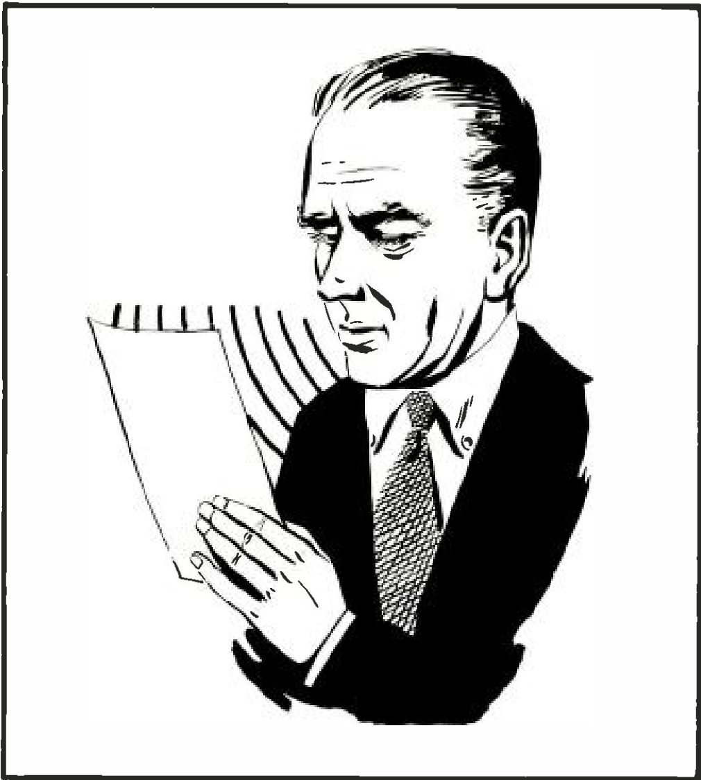
Fig. 2-1. Speaking directly at a sheet of paper will cause it to vibrate exactly as does the diaphragm of a microphone.
