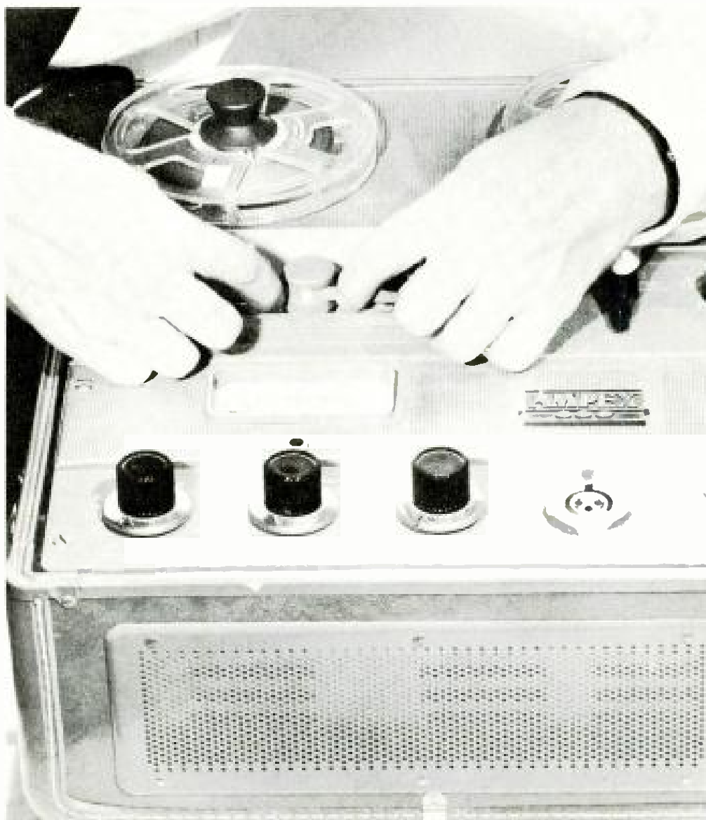
Fig. 9-14. A single tone of short duration, such as a hand clap, may be removed by holding the tape against the recording head for a moment, then gradually drawing it away.
