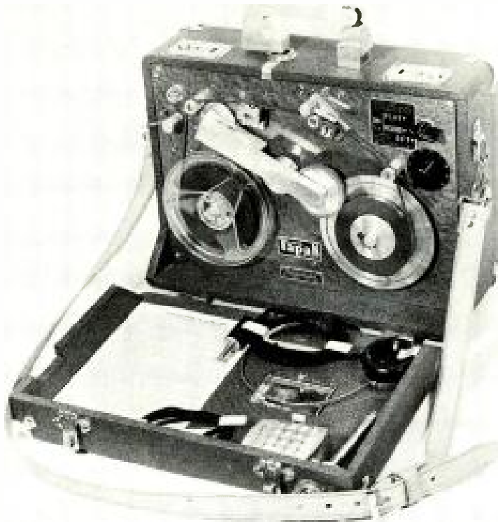
Fig. 13-1. The Travis Tapak, a battery-operated portable tape recorder. (Photo Courtesy of Broadcast Equipment Specialties Corp.)
