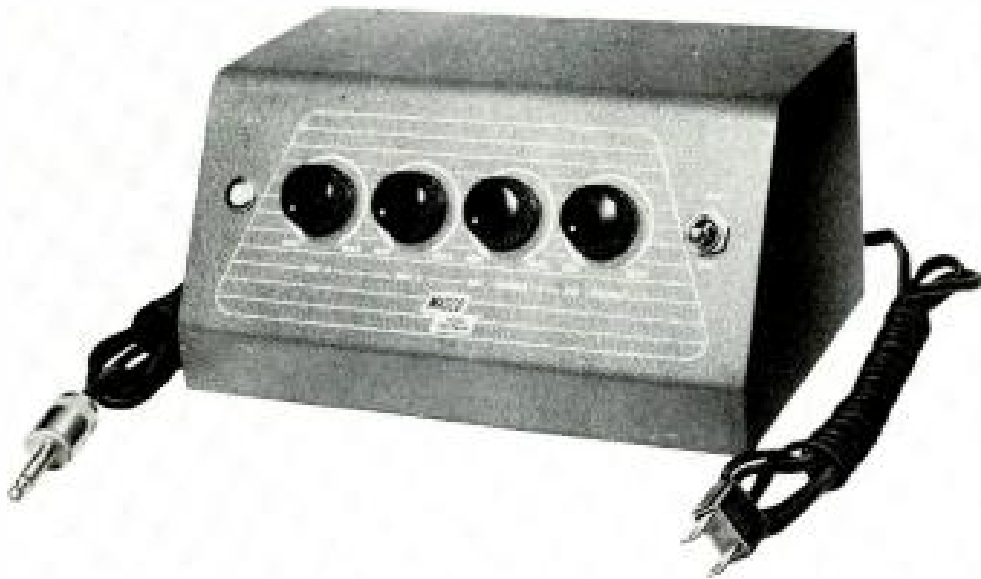
Fig. 6-11. Two electronic mixers which can be used to mix and fade microphone, radio tuner, phonograph, and the like. (Photos Courtesy of Pentron Recording Corporation and Masco Sound Systems.)
