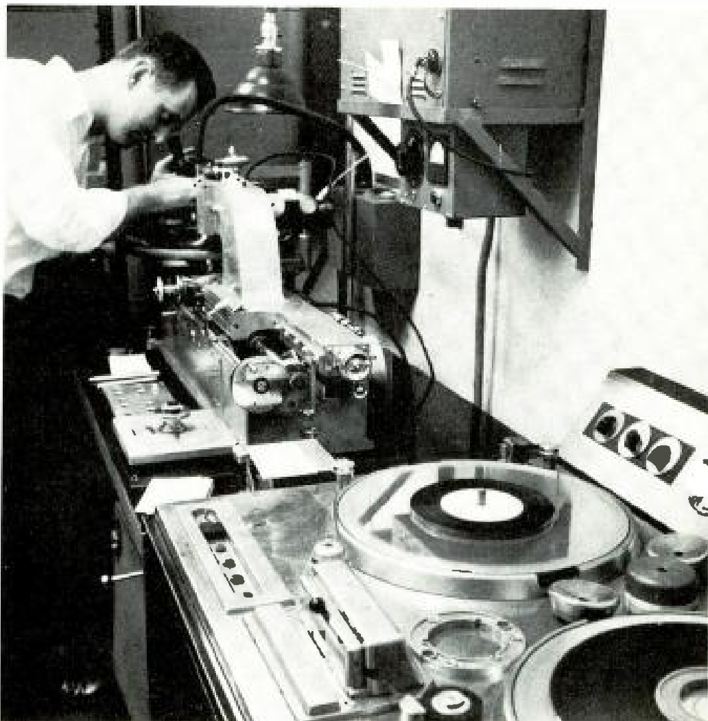
Fig. 1-1. Transferring recorded sound from magnetic tape to a master disc. (Photo Courtesy of Columbia Records, Inc.)
