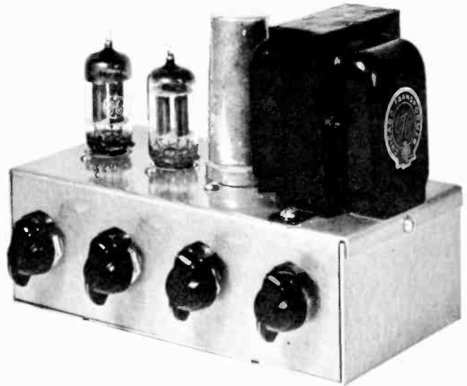
Fig. 4. Three-element bass-boost circuit with self-contained power supply.
