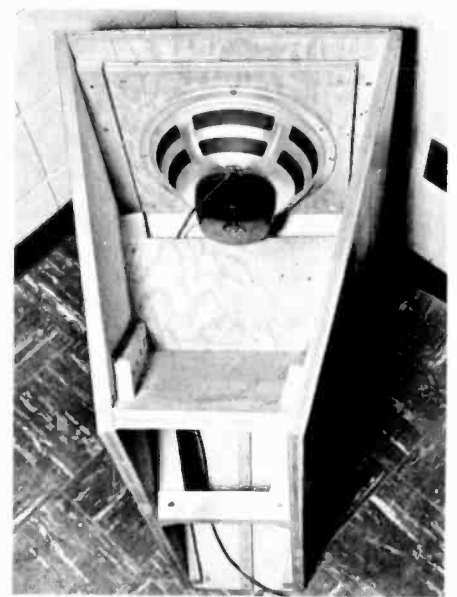
Fig. 3. This view of the enclosure turned around from its normal position, was taken from above and behind. It is useful in showing many details, though somewhat deceptive from a photographic standpoint. To avoid misunderstanding, remember that the side walls are rectangular, the top parallel to the floor.
