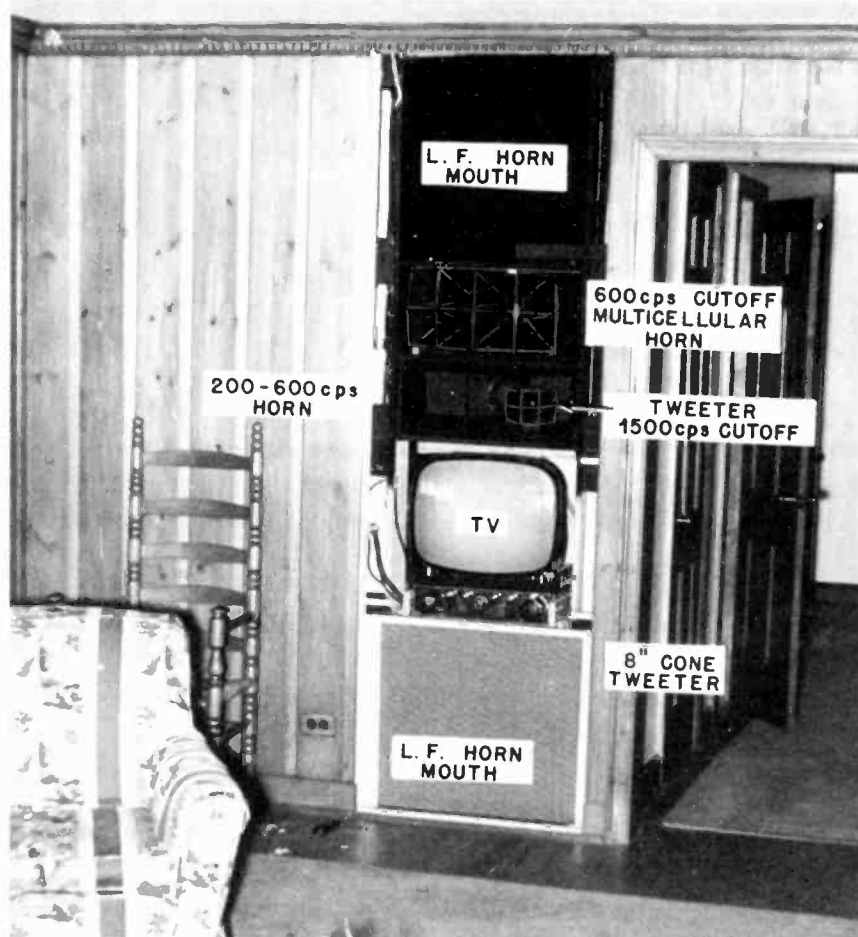
Fig. 1. The finished enclosure is mounted in a closet with the divided horn exhausting into the listening area. Between the two sections is the TV receiver. The upper section will be covered with a grill similar to that over the lower section.
