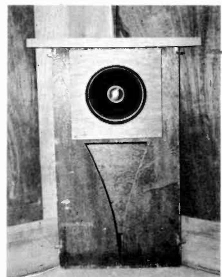
Fig. 9. Semi-finished cabinet with loudspeaker in place on its mounting panel. Note brackets on edges of front panel for mounting the trimming frame.
