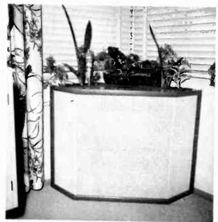
Fig. 2. Closeup of the mid- and high-frequency speaker section in the corner cabinet.
