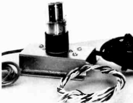
Fig. 3. Adapter chassis used with electronic organ, showing simple "add-on" unit which may be employed with tuner or any other sound source.
