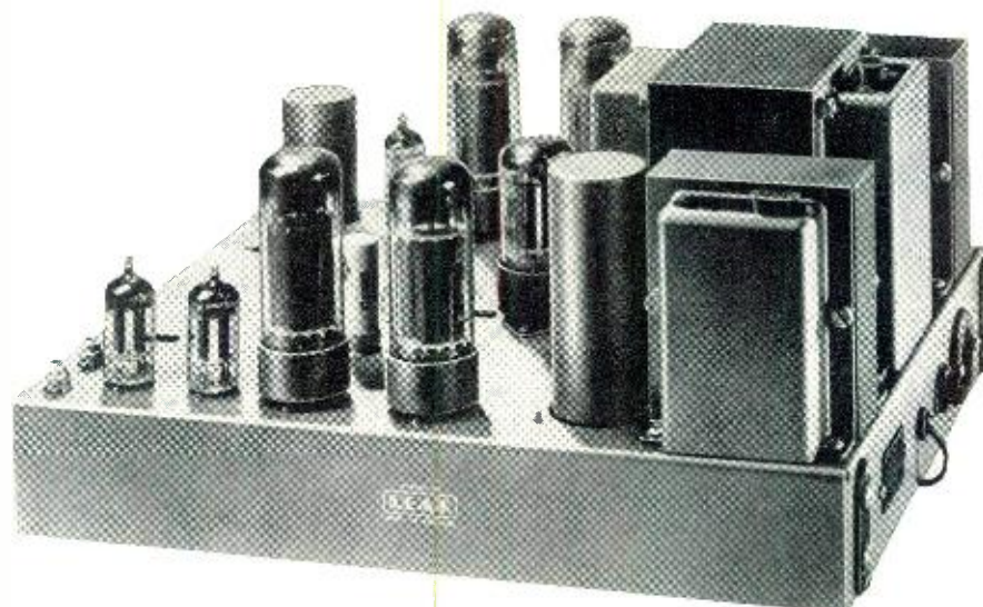
Fig. 4. The Leak "Stereo 50" power amplifier, a pair of 25-watt amplifiers on the same chassis.
