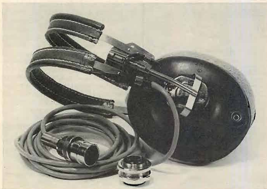
Fig. 1. Modified phones showing wiring method, 4-pin plug, and matching connector.
