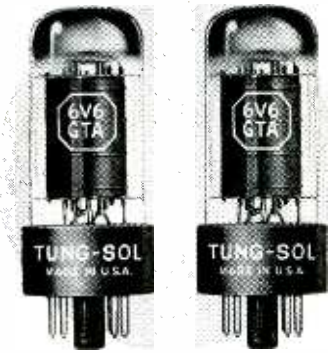
6V6GTA Bantam beam power amplifier with high power sensitivity and high power output with low supply voltages. Two in push-pull up to 14 watts.
