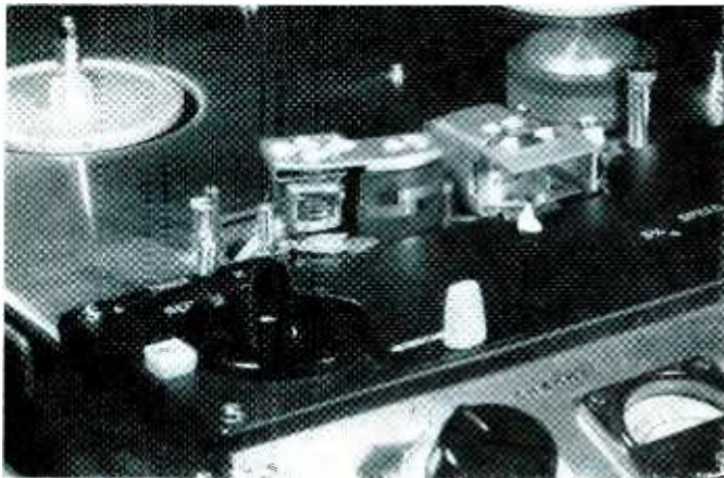
Fig. 2. Head assembly of Model 555-A4 Stereorecorder showing position of four-track head.
