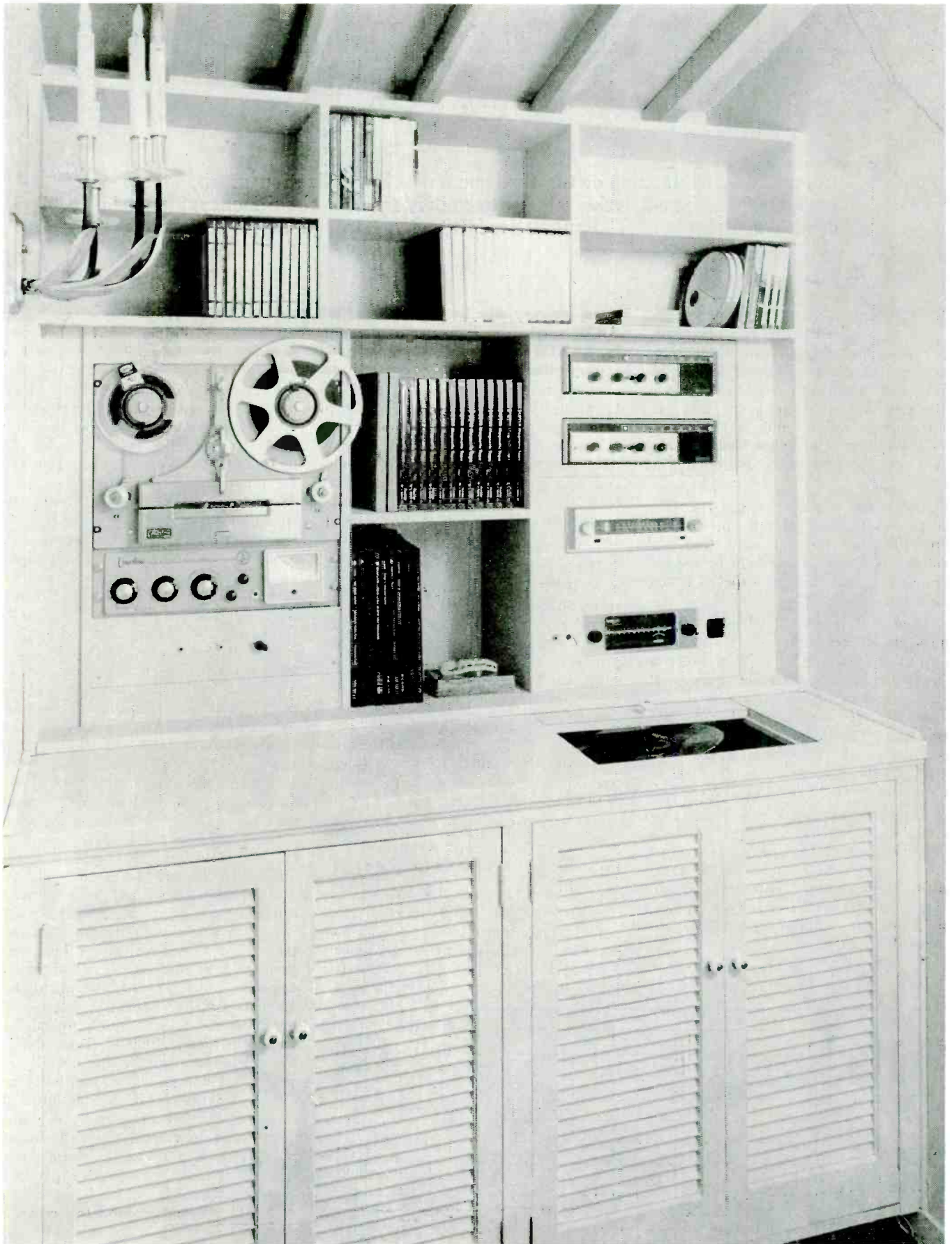
"Hi-Key Hi-Fi" is the title given this picture by Max Eckert, P. O. Box 535, Sepulveda, California—an installation designed and executed by Robert de Horoch, Hollywood. Located in the entry hall, all controls are at eye level with shelves for tape and record storage. Speakers are in living room adjacent—two James B. Lansing D130's, two University HF206's, two University crossover networks. Concertone Series 20 tape recorder, Thorens CD43N changer, Sherwood S-2000 AM-FM tuner, and Harman Kardon A-400 FM tuner furnish the sources to National amplifiers and preamplifiers.
