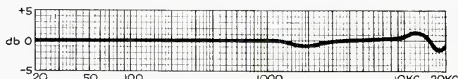
TYPICAL FREQUENCY RESPONSE OF VR II CARTRIDGE MEASURED ON A CONSTANT VELOCITY BASIS
