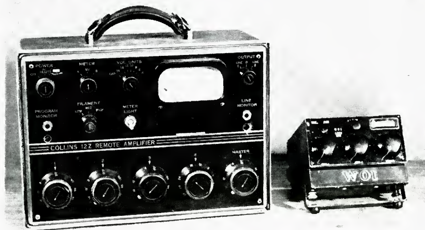
Fig. 1. The transistorized remote unit developed at WOI shown alongside a conventional tube-type Collins 12Z remote amplifier.
