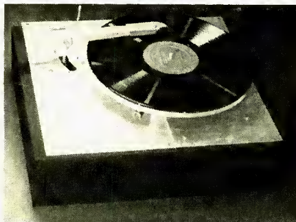
Fig. 4. Three-quarter view of device in operation. Notice slot to accommodate the movable pickup arm mount post.
