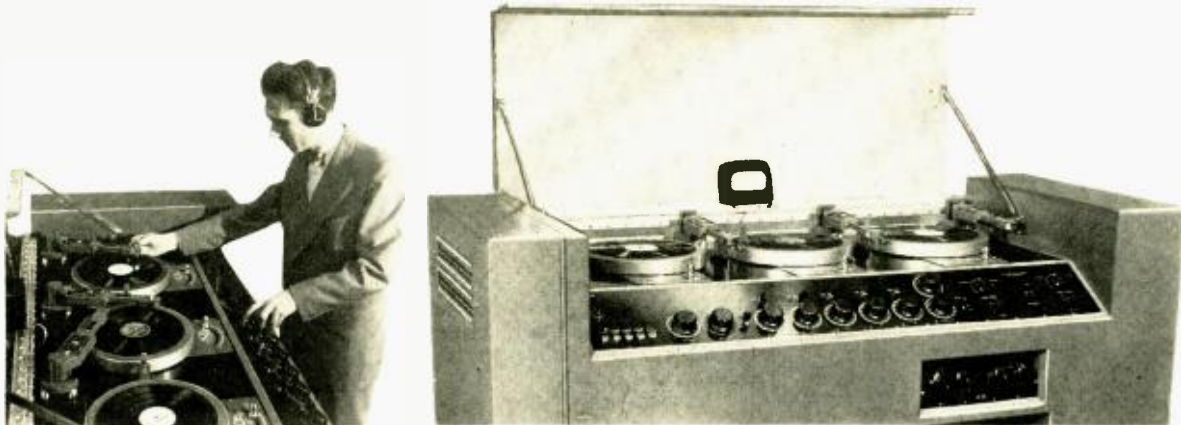
Fig. 1. Two views of the sound-effects console. Left, from the front to show the general arrangement, and in use, at the right, indicating the convenient placement of controls and pickup arms.
