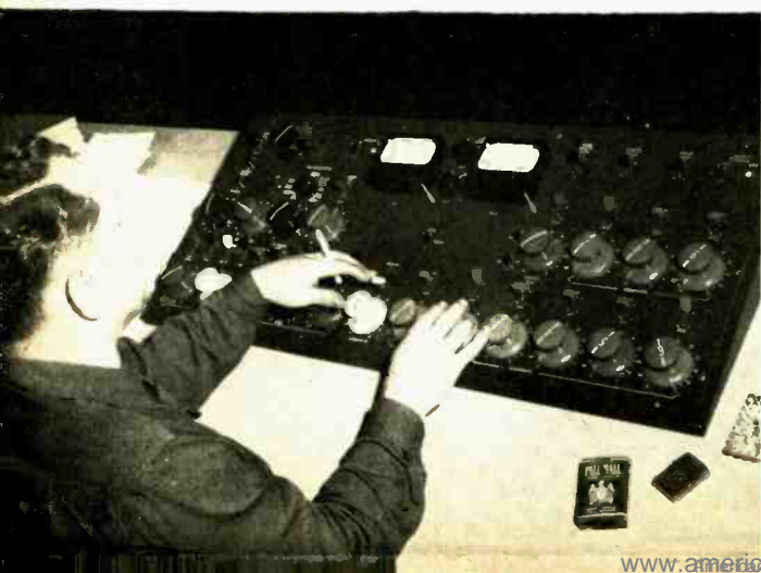
Color coding of knobs and switches facilitates quick handling by the engineer, while the four-inch elevation of the back provides maximum visibility of the studio below.
