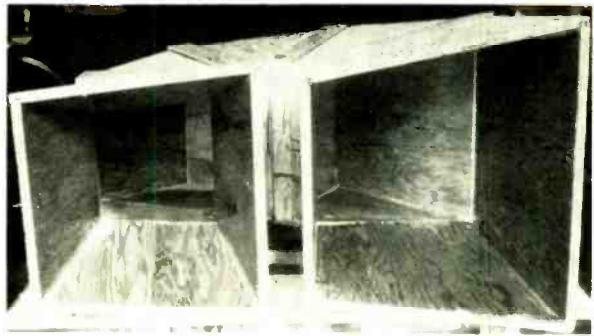
Fig. 2. Front view—left is the speaker housing, with the horn mouth shown at the right. The two are connected by a semicircular horn.
