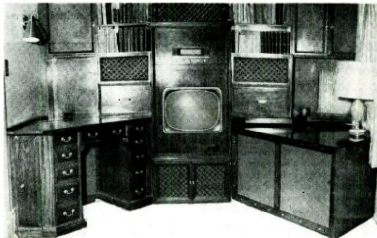
The semicircular exponential horn enclosure as part of the author's music unit. It is detached to avoid acoustic feedback. Behind left and right grill-drawer compartments are phono and professional tape deck. Center top grill conceals separate TV speaker in a ventilator shaft, and tuner front end controls a remote third speaker. Built-in desk balances speaker enclosure. The center section and speaker horn enclosure are on casters and roll out for maintenance. Subassembly of desk, and left and right halves of shelves are screwed and dry-doweled for ready disassembly of entire unit for possible future reinstallation. Unit constructed by Fred Nelson, Kings Park, N. Y.
