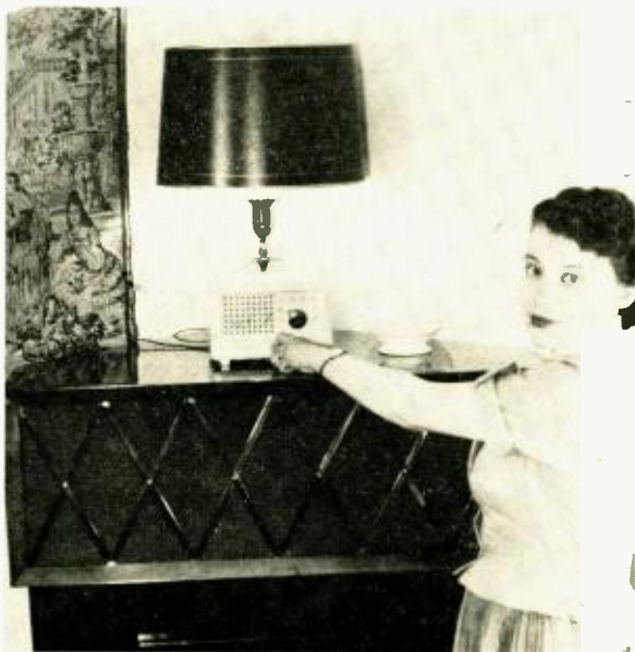
Fig. 2. The simplest kind of a.c.-d.c. receiver serves as an inexpensive tuner of good quality for AM reception.
