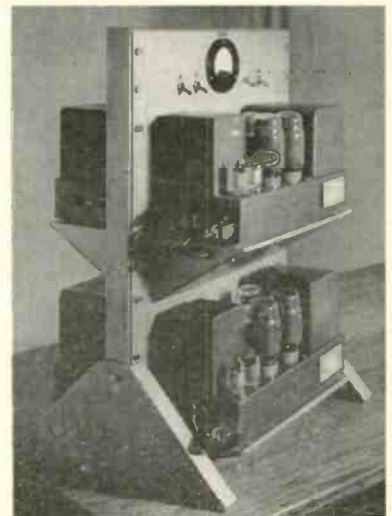
Fig. 3. The four standard QUAD amplifiers were mounted on this small rack.
