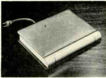
Fig. 56. The Rauland "Libretto"—the backbone of the "book" hinges open to give access to the controls.
