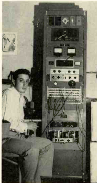
The elaborate system owned by Robert Schwartz, '57, of Burton House, includes a Fisher FM tuner, Master Audio Control, and 50-watt amplifier, and a Heathkit preamp and a 6-watt Williamson amplifier—the latter being used only for cueing. Bob's interest is mainly in popular music, but when he feeds the lines, the quality is professional.
