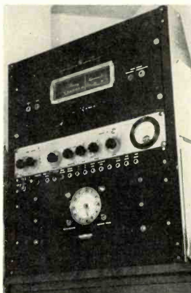
Author's rack contains a Browning RV-10B tuner, modified McIntosh C-104 preamp, Williamson amplifier, Sessions timer, VU meter, patch panel, and controls for noise suppressor. Line jacks are closed circuit, with contacts normalised to feed regular "network."
