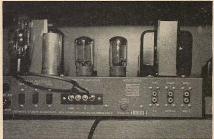
Fig. 1. In this "switchboard of home entertainment, six input sockets give your audio system extreme flexibility, accommodating Pickering pickup in Mag-1, GE and Audax in Mag-2, crystal in Xtal; in addition, there are radio, television, and tape recorder inputs.
