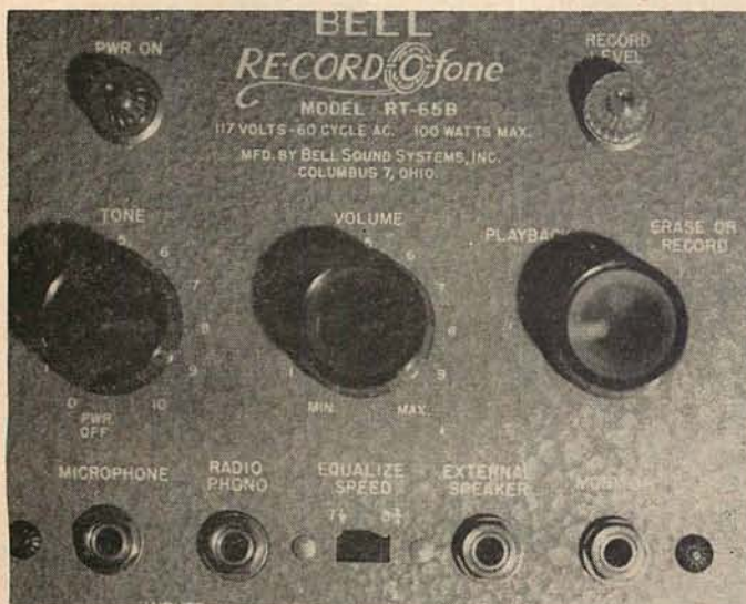
Fig. 2. Inputs on the face of this tape recorder handle microphone, radio, and phonograph. Output marked External Speaker feeds to amplifier input marked Tape in Fig. 1.
