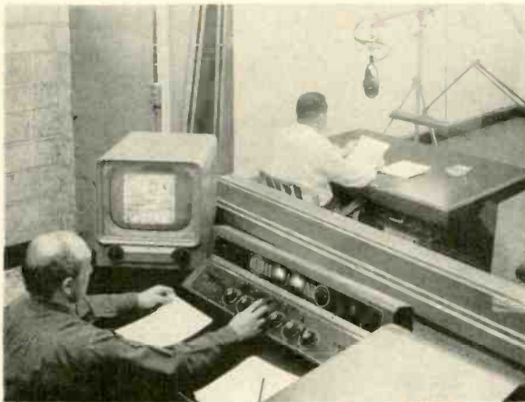
Typical studio application of the new volume visualizer, using a conventional scope as the indicator.
