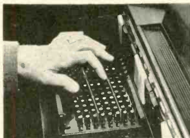
Fig. 2. The chord section is operated by 96 buttons, providing eight chords for each of the twelve keys in an octave.
