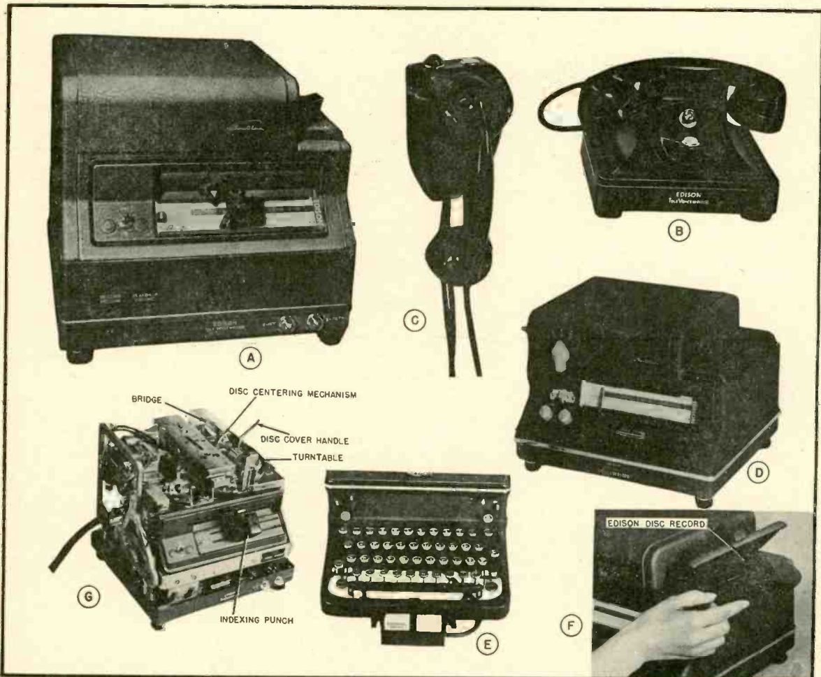
Fig. 9. The TeleVoicewriter and related equipment: (A), recorder; (B), executive desk station; (C), alternate wall station; (E), secretarial start-stop-backspace control mounted on typewriter; (D), secretarial transcribing instrument; and (F), method of placing disc in recording position; (G), the recorder with the outer case removed.
