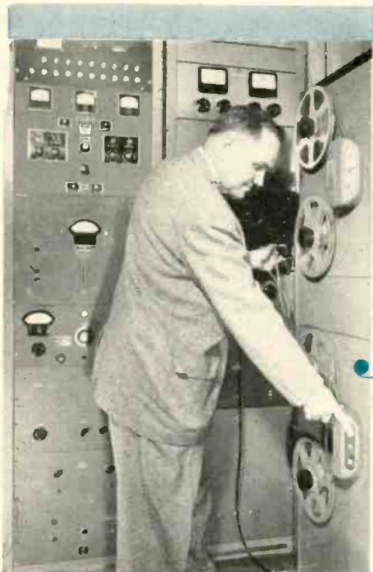
An Ampex Automatic Station now in operation at KEAR in San Mateo, California. It sustains the evening programs on tapes prepared by the daytime staff.
