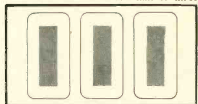
Fig. 2. Three rectangular c-r tubes arranged for presentation of level information on three channels simultaneously.
