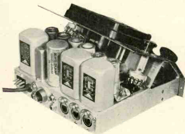
Fig. 2. View of the chassis removed from the case to show new transformers and new mounting of the selector switch.
