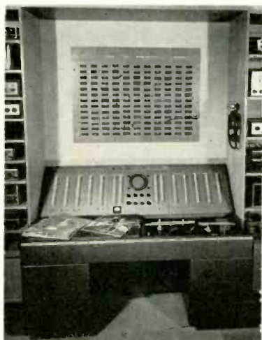
Close-up of the "Auditioner"—which is a playing desk with several turntables combined with switching facilities for various amplifiers, tuners, and speakers. Above the control panel is an indicator which shows the equipment in use.
