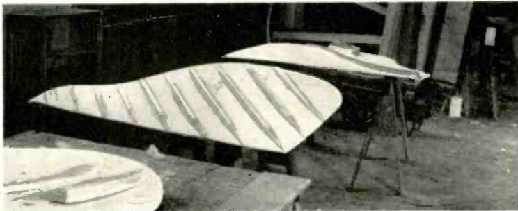
Fig. 4. Details of the soundboard for a small grand piano. (Courtesy The Baldwin Piano Co.)
