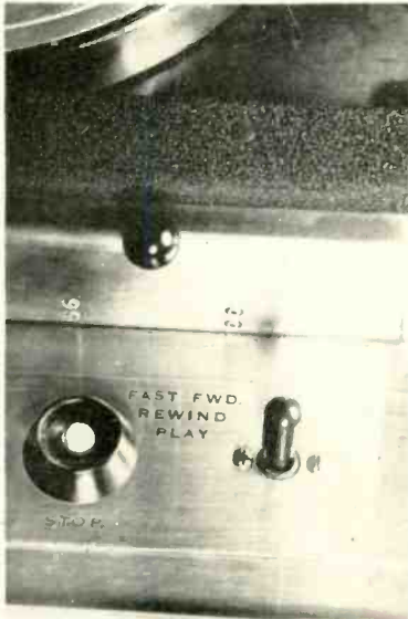
Fig. 1. Cam lever switch mounted on the front panel of an Ampex 300 tape recorder in place of the rotary switch. Switch-handle motion is forward and backward, but name plate had not been changed.
