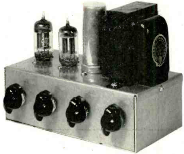
Fig. 4. Three-element bass-boost circuit with self-contained power supply.
