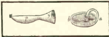
Fig. 4. Artificial hearing mechanism. The combination of horn and diaphragm is prophetic of 19th century phonograph design.
