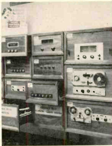
Fig. 3. One section of the equipment rack, which consists of separate drawers faced with finished hardwood; panels are simply pulled forward to permit inspection of the equipment. Note name panels which are illuminated when the equipment is being demonstrated
