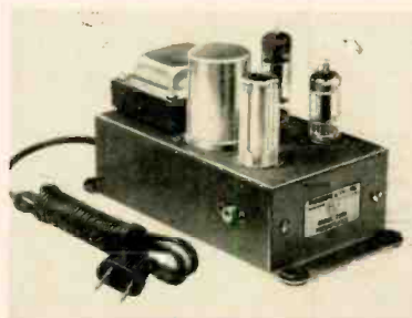
Fig. 4. Another self-powered preamplifier is the Pickering, Model 230H, with vibration-reducing rubber grommets for mounting.
