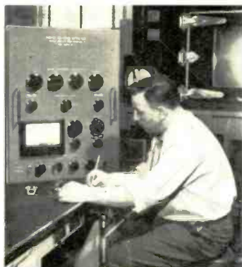
Q meter measurements on low frequency coils
