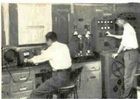
Testing modulation transformer under operating conditions
