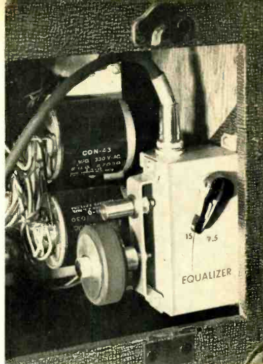
Fig. 7. Equalizer in its shield can is mounted inside the recorder case, and supports bracket for idler and capstan sleeve.
