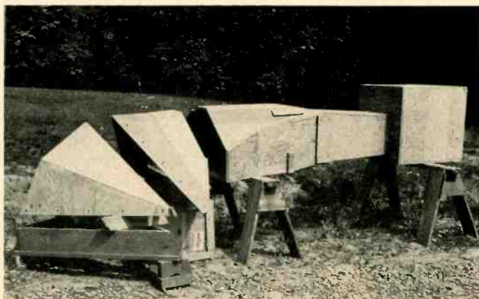
Fig. 3. By constructing the horn in sections, it is possible to handle it without the aid of a crane.
