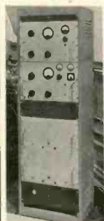
Double installation of Gramplan Amplifier with Power Supply
