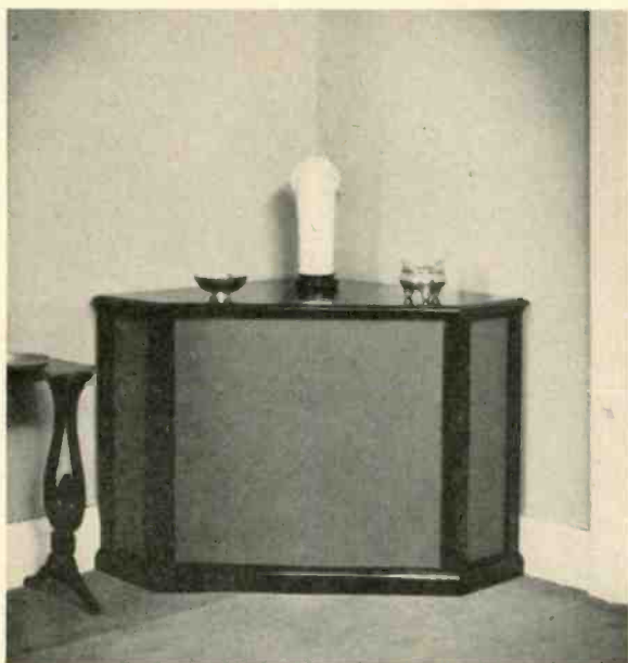
Fig. 6. Corner cabinet design employing two-path rear loading and direct-radiation from front of cone.
