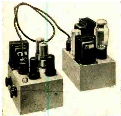
Fig. 1. Separate chassis for the amplifier and power supply simplify mounting in many applications.
