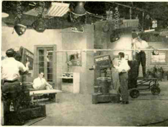
Fig. 5. A flexible and easily operated boom stand is an invaluable piece of TV studio microphone pickup equipment.
