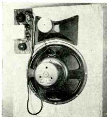
Fig. 8. Baffle with two-cell Racon horn and 15" Jensen cone and dividing network for 1,200-cps crossover frequency.
