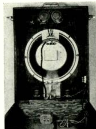
Fig. 4. Experimental assembly of 12" cone and University Model 4402, with dividing network and impedance-matching input transformer.
