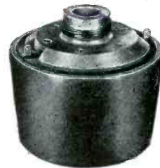
NEW SPECIAL PM HORN UNIT , having Alnico V magnet ring, completely watertight, housed in a heavy aluminum spinning. Provides extremely high efficiency reproduction with minimum input. Handling capacity 35 watts continuous, 60 w. peak.
